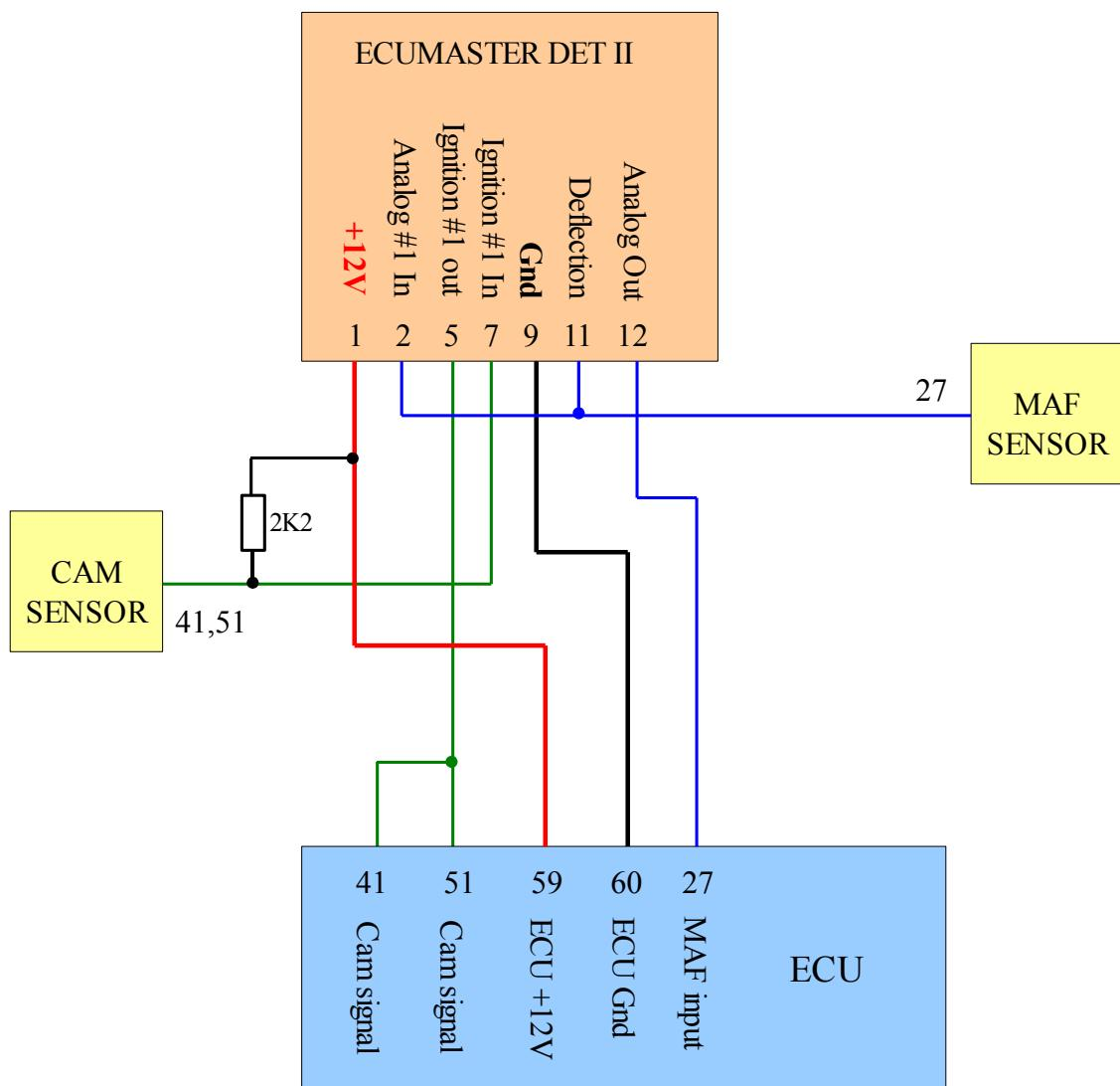
**Comment:** Wires from pin 41 and 51 are connected together about 30cm from ECU. Connect DET 2 ignition input / output to the common wire of these pins. It is suggested to use external map sensor as deflection.
